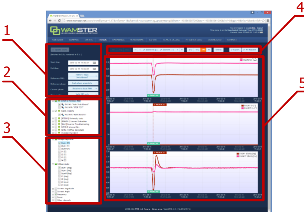
Figure 6.15: Trends page can be used to view and compare measurements during different time periods
