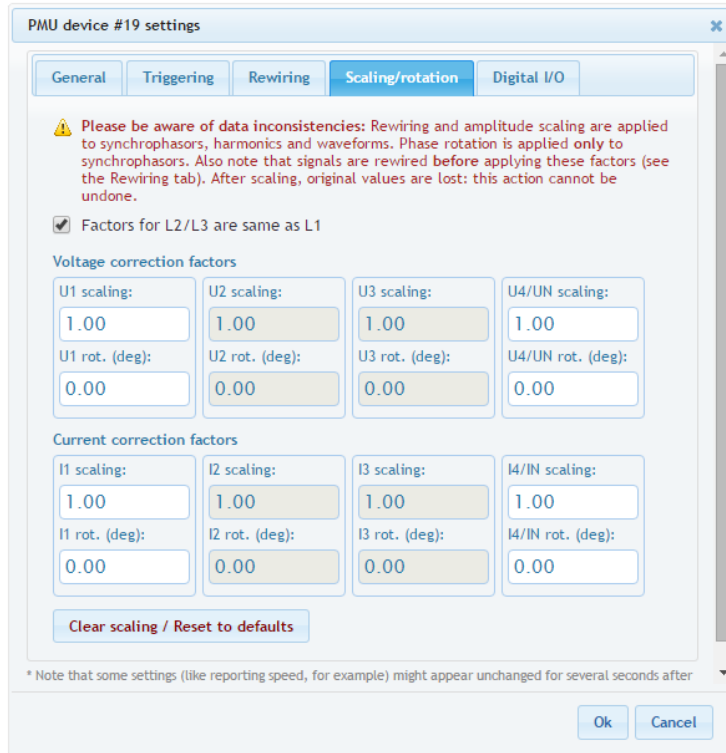
Figure 6.8: Scaling/rotation tab can be used to further correct measurements after rewiring
