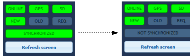
Figure 6.23: If the remote instrument is in a different menu than the one shown on the web page, remote status will change to "NOT SYNCHRONIZED"
