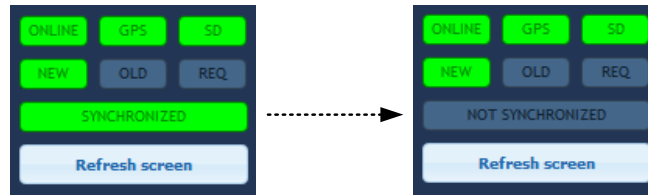
Figure 6.11: If the remote instrument is in a different menu than the one shown on the web page, remote status will change to "NOT SYNCHRONIZED"
