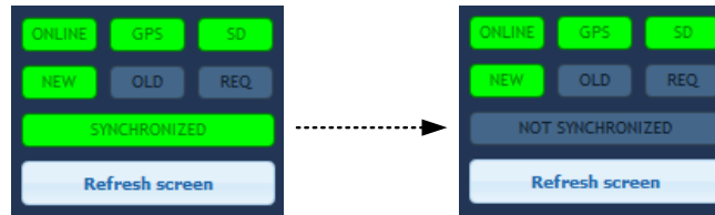
Figure 6.13: If the remote instrument is in a different menu than the one shown on the web page, remote status will change to "NOT SYNCHRONIZED"
